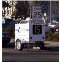
**Speed Watch Radar Trailer:** a self-contained speed monitoring radar trailer, placed at the roadside, displaying the speed of on-coming vehicles. Citizens may request placement locations.
